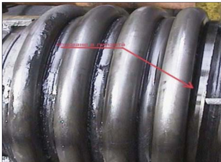
The red arrow indicates the crack in the heat exchanger's compensator (Fig. 9).
